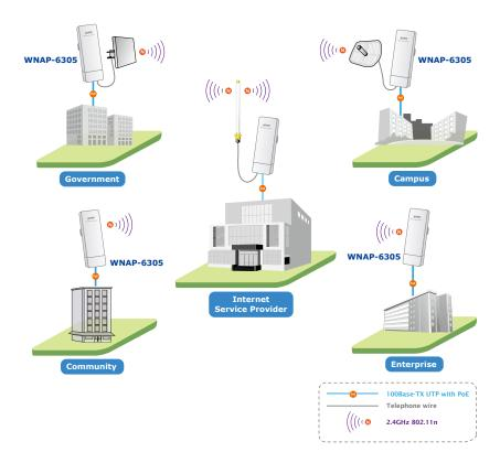
With a built-in SMA-type antenna connector and high output power with multiple adjustable Tx controller, the WNAP-6305 provides higher coverage and longer distance wireless connection, and also allows CPE users to easily install and adjust the suitable value in appropriate locations. The WISP mode supported enables CPE users to connect to Internet via local WISP provider.
